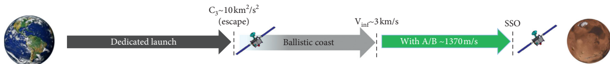
FIGURE 9: Launch and transfer scenario for the Mars Science Orbiter (MSO) mission.
