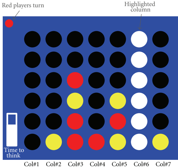
FIGURE 2: P300-based BCI “Connect Four”. Black disks represent the empty places. Yellow and red disks correspond to player P1 and player P2 pieces, respectively. The column made of white disks represents a flashed column.
