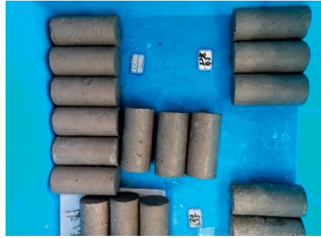
FIGURE 5: The demoulded cement modified slurry (CMS) sample.
