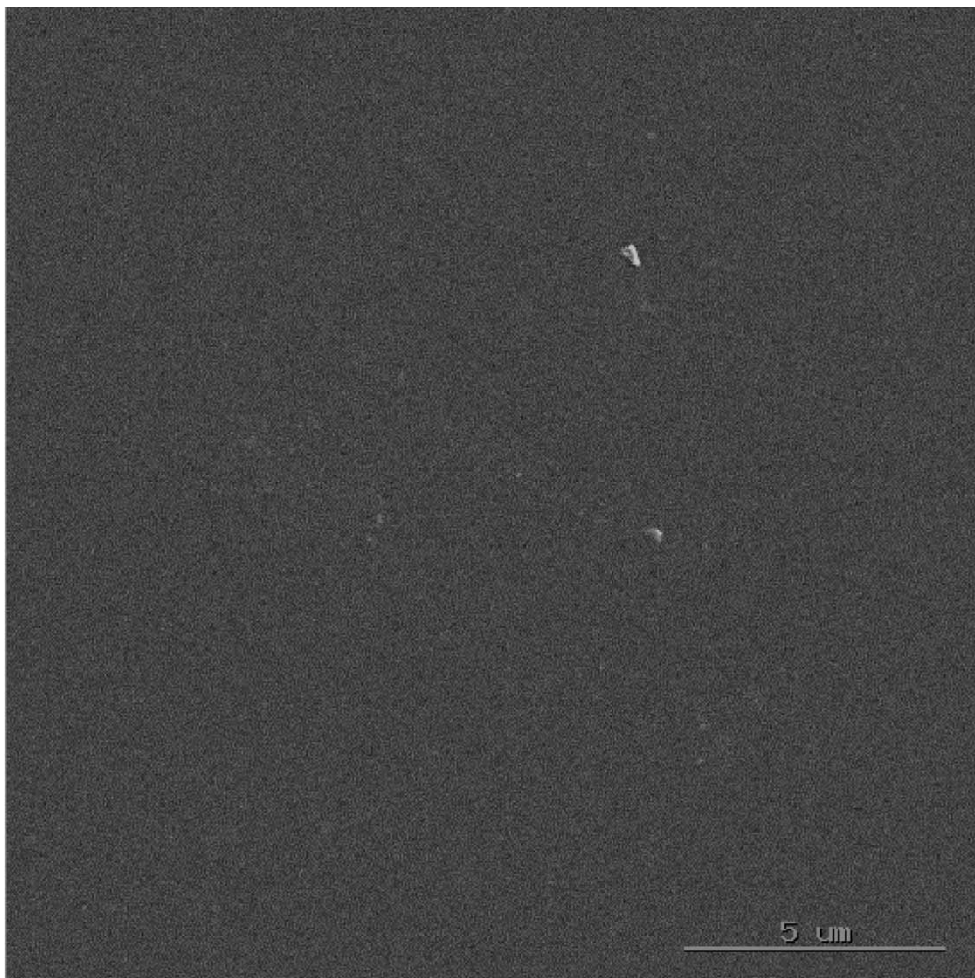
FIGURE 9 SEM for quenched sample of n-Si from 600 °C with scale of 5 μm.
