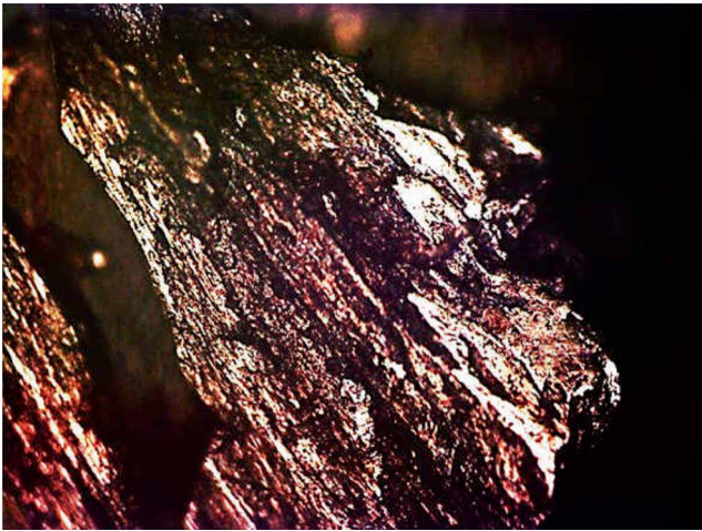
FIGURE 14: Metal squeeze out due to high load (2300 N) 0.5% GNPs-NO.
