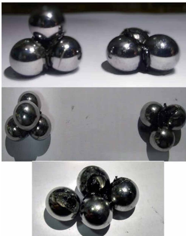
FIGURE 10: Steel balls after extreme pressure test at the seizure load.
