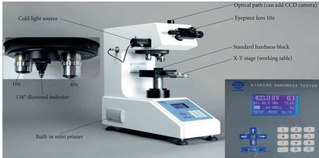
FIGURE 6: HVD-1000 MP micro-Vicker hardness tester.
