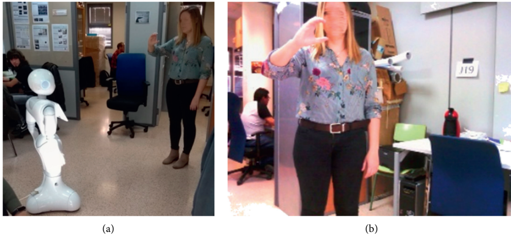
FIGURE 2: Sample of image capture. (a) Pepper capturing images while person signing. (b) Image captured by Pepper for the dataset.
