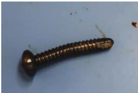
FIGURE 8: The compression screw removed after bone union was bent because of the compression force.
