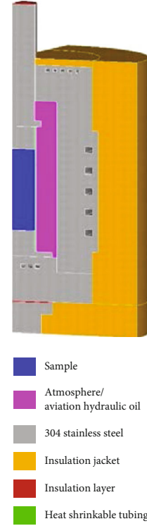
FIGURE 8: Finite element model of the triaxial cell and its internal components.
