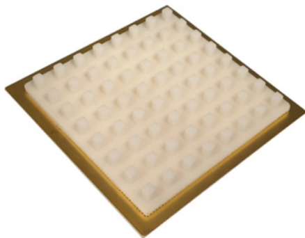
FIGURE 9: Top view of the 8 \times 8 DRA array proposed in [68].
