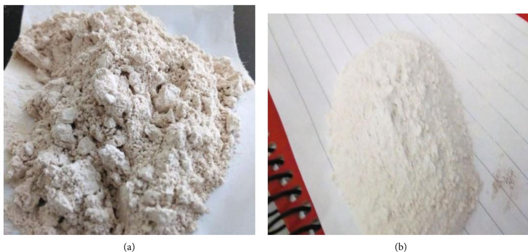
FIGURE 2: Photo images of (a) kaolin clay before and (b) after purification.
