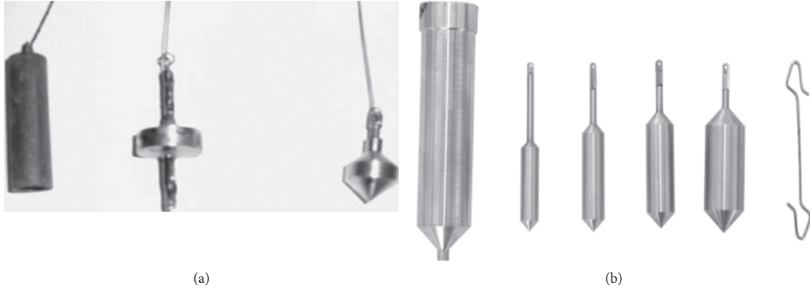
FIGURE 4: Shape of viscometer rotor. (a) Traditional rotor shape. (b) The rotor shape is selected in this paper.
