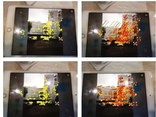
FIGURE 4: Feature point tracking effect of the KLT optical flow algorithm.
