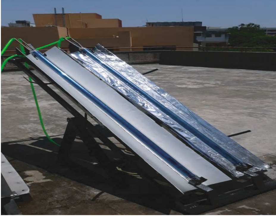
FIGURE 3: CPC with aluminum foil and Mylar.
