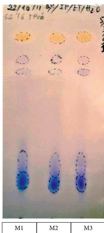
FIGURE 2: HPTLC of reference samples M1, M2, and M3 (50-month-old) developed in system A— butanol/isopropanol/ethanol/water (5:3:2:1 v/v).
